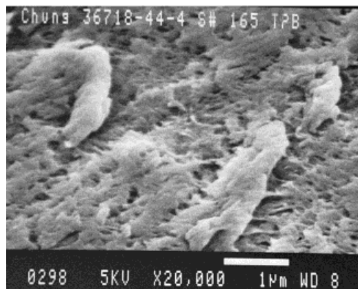
Figure 6 SEM pictures of the cross-section and external surface of fibers precipitated in 10°C (internal coagulant = 80/20 acetone/water, external coagulant = 20/80 DMAc/MeOH, 2.54 cm air-gap). Magnification: \times 750 (top) and \times 20,000 (bottom).
