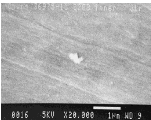
Figure 15 The effect of external coagulant, 80/20 acetone/water, on wet-spun fiber morphology (internal coagulant = water). Magnification: cross section (top) \times 750 and outer skin (bottom) \times 20,000 , \times 10,000 (right).
